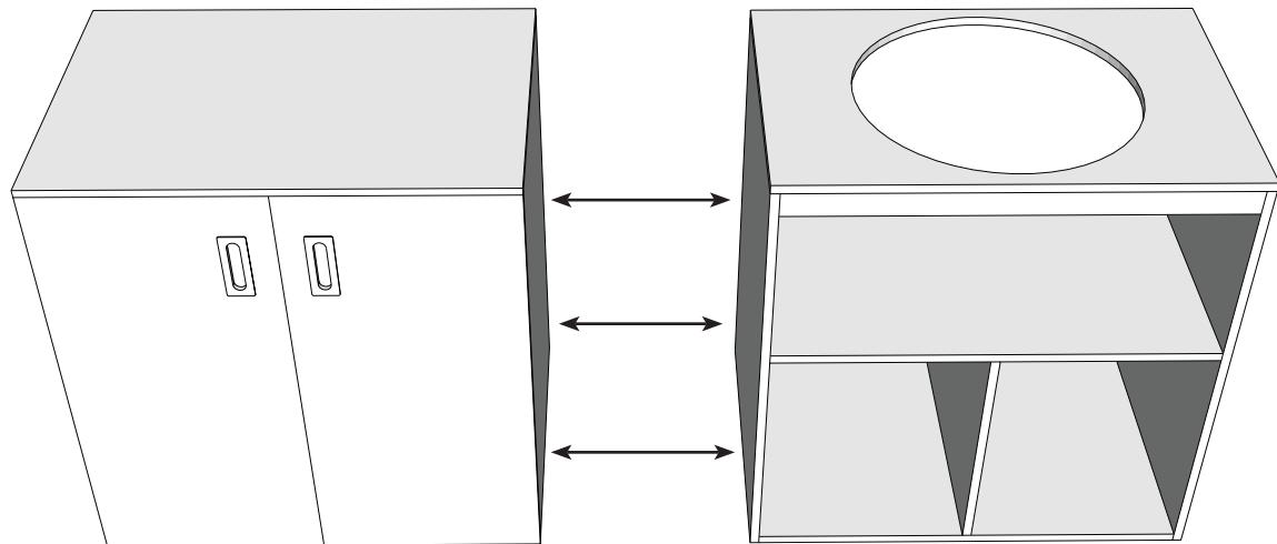
Drill holes in the prepared places - drill bit 5 mm
